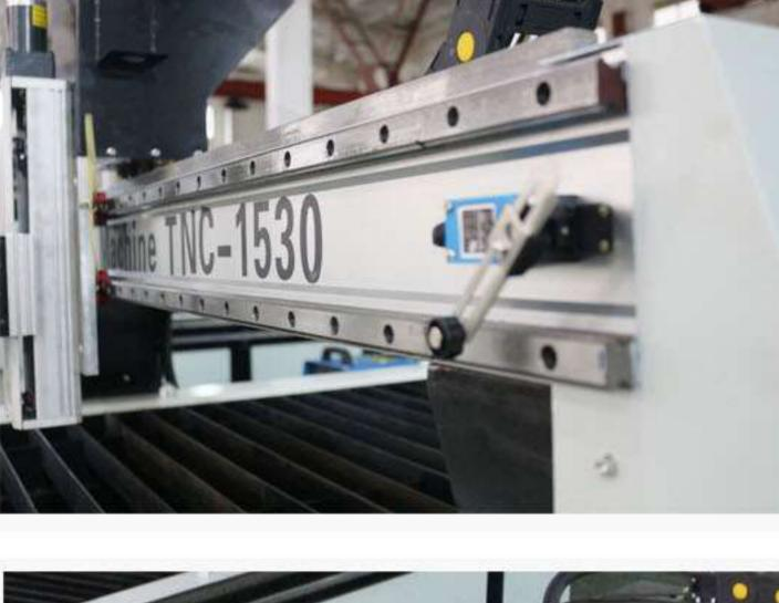
1)Y axis adopt double linear guide rail, gear and rack transmission is more stable.
