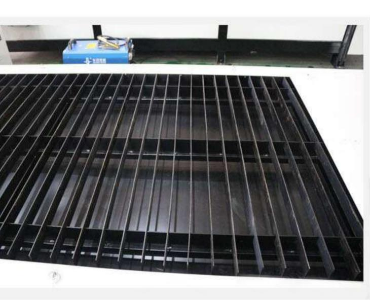
Closed environment-friendly bottom channel (water filling) and dust treatment system can timely and effectively discharge dust to ensure the staff health
